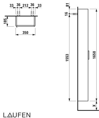
X = The exact hight must be set during installation.
