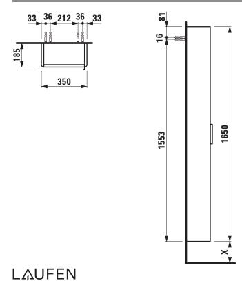
X = The exact hight must be set during installation.
